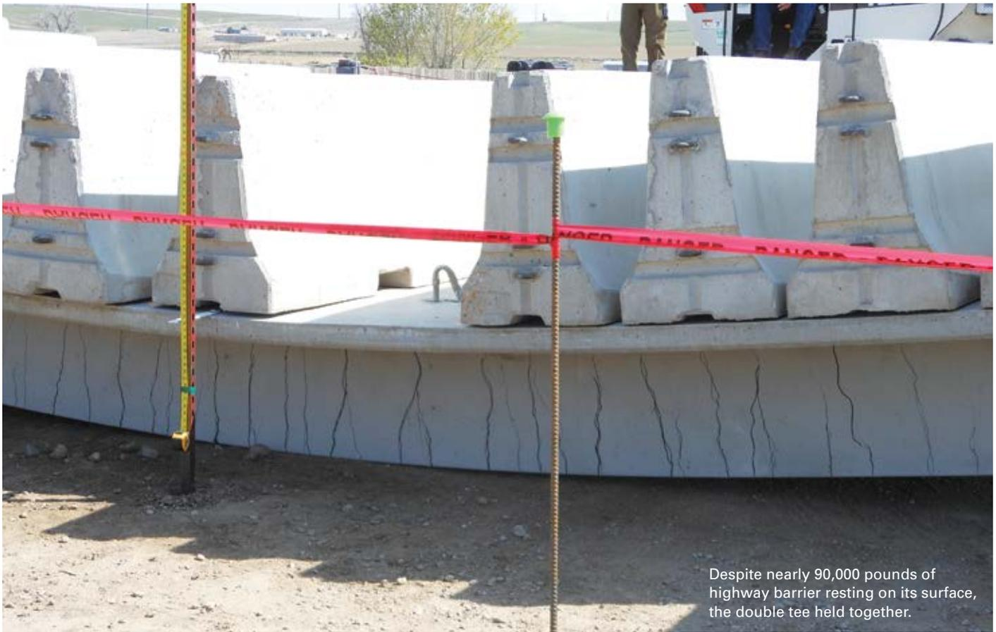
Despite nearly 90,000 pounds of highway barrier resting on its surface, the double tee held together.
